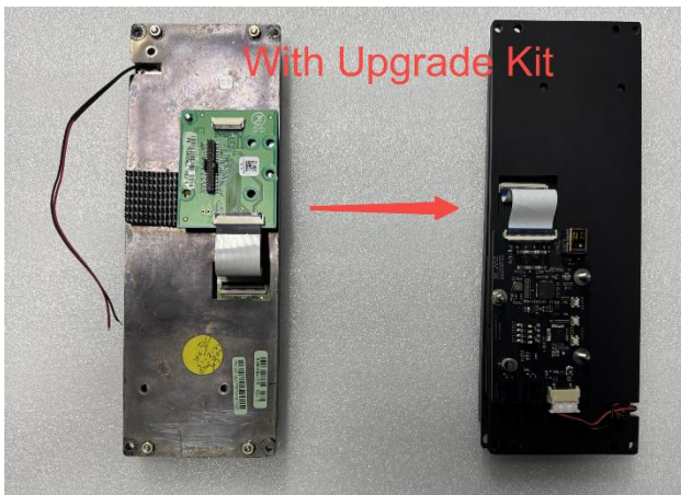
6.2" IGT Player Tracking Display with 4-Wire Resistive Touchscreen
